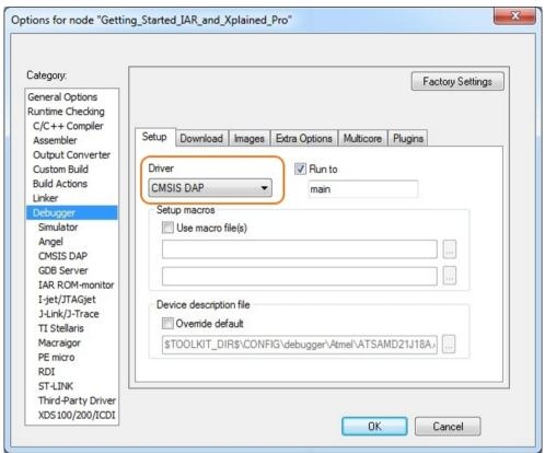
Figure 5-3. Configure Flash Loader
