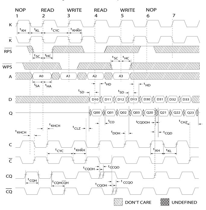
Figure 5. Read/Write/Deselect Sequence <sup>[29, 30, 31]</sup>
