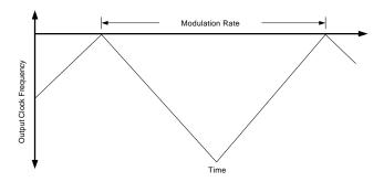
Figure 3. Spread Spectrum Triangle Waveform
