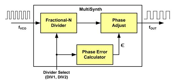
Figure 2. Silicon Labs' MultiSynth Technology
