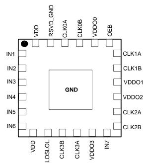
**Note:** Center pad must be tied to GND for normal operation.
