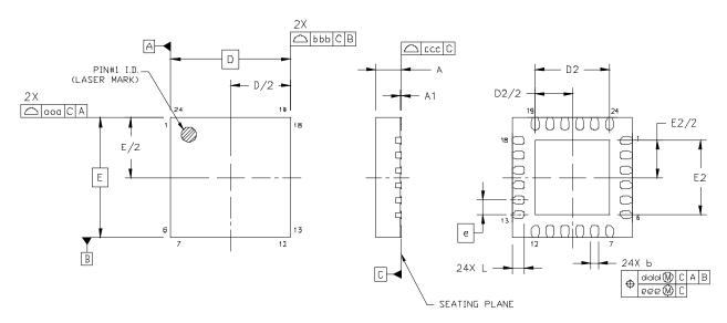
Figure 4. 24-Lead Quad Flat No-lead (QFN)
