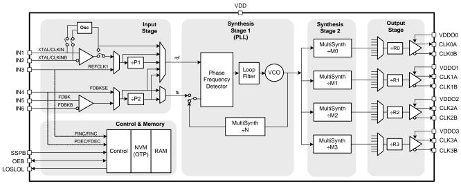
Figure 1. Si5334 Block Diagram
