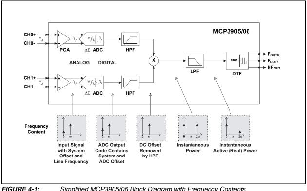
Simplified MCP3905/06 Block Diagram with Frequency Contents.
