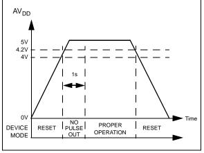
FIGURE 4-3: Power-on Reset Operation.
