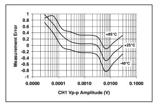
FIGURE 2-6: Measurement Error, Gain = 32, PF = 0.5.
