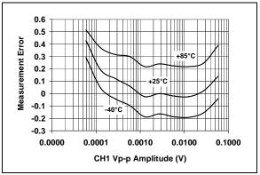
**FIGURE 2-4:** Measurement Error, Gain = 8, PF = 0.5.
