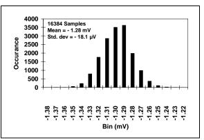
**FIGURE 2-14:** Channel 0 Offset Error (DC Mode, HPF Off), G = 16.
