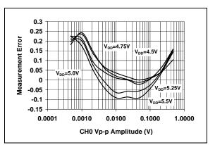
**FIGURE 2-16:** Measurement Error vs.  $V_{DD}$ , G = 16, External  $V_{REF}$ .
