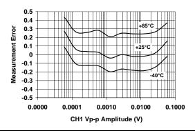
FIGURE 2-1: Measurement Error, Gain = 8, PF = 1.
