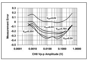
**FIGURE 2-15:** Measurement Error vs.  $V_{DD}$  (G = 16).
