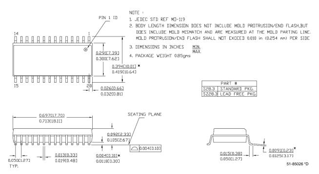
Figure 20. 28-Lead (210-Mil) SSOP
