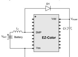
Figure 8. Basic Switch Mode Pump Circuit
