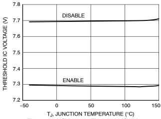
Figure 11. NCV887801 Threshold IC Voltage vs. Temperature
