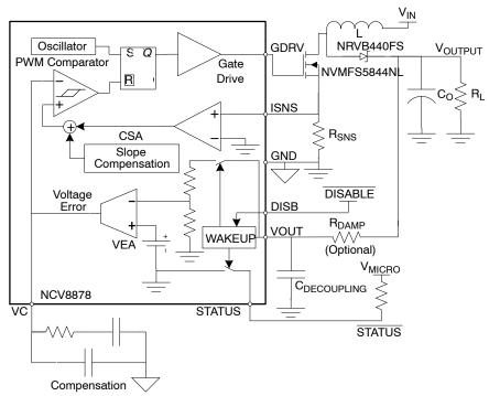
Figure 13. Current Mode Control Schematic
