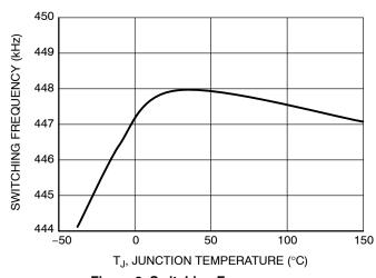
Figure 9. Switching Frequency vs.
