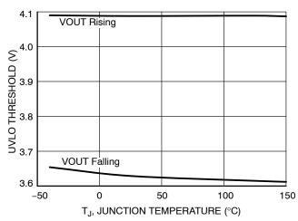
Figure 10. UVLO Threshold vs. Temperature
