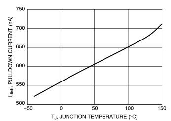
Figure 12. DISB Pulldown Current vs. Temperature
