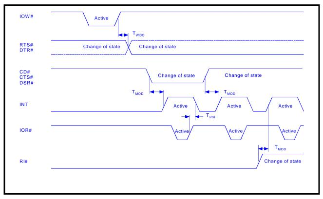
FIGURE 15. 16 MODE (INTEL) DATA BUS READ TIMING
