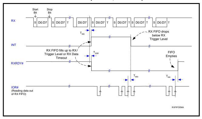
FIGURE 23. TRANSMIT READY & INTERRUPT TIMING [FIFO MODE, DMA MODE DISABLED] FOR CHANNELS A & B
