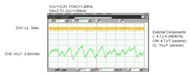
18. Please note the inductance value of the coil. The IC may enter unstable operation if the combination of ambient temperature, setting voltage, oscillation frequency, and L value are not adequate.
