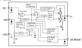
NOTE: The signal from CE/MODE Control Logic to PWM/PFM Selector is being fixed to "L" level inside, and XC9235 series chooses only PWM control.
