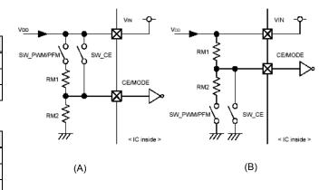
Intermediate voltage can be generated by RM1 and RM2. Please set the value of each R1, R2, RM1, RM2 from few hundreds k to few hundreds M . For switches, CPU open-drain I/O port and transistor can be used.
