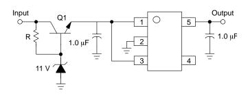
Figure 24. Input Voltages Greater than 12 V
