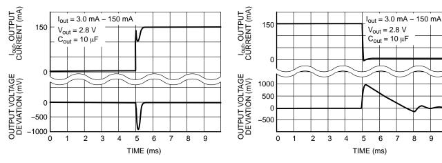
Figure 12. Load Transient Response ON
