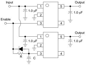
Figure 23. Delayed Turn-on
