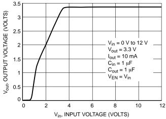
Figure 18. Output Voltage versus Input Voltage
