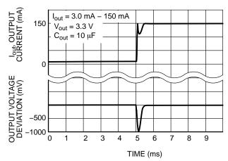
Figure 14. Load Transient Response OFF
