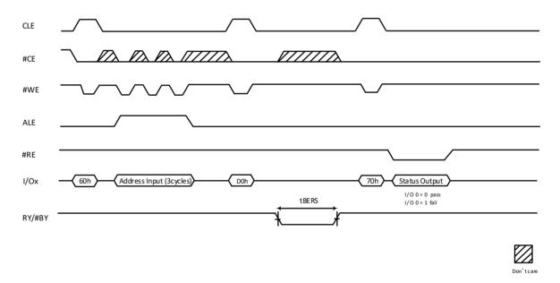
Figure 9-18 Block Erase Operation
