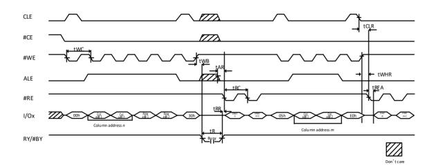
Figure 11-9 Random Data Output Operation
