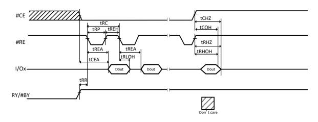
Figure 11-5 Serial Access Cycle after Read (EDO)
