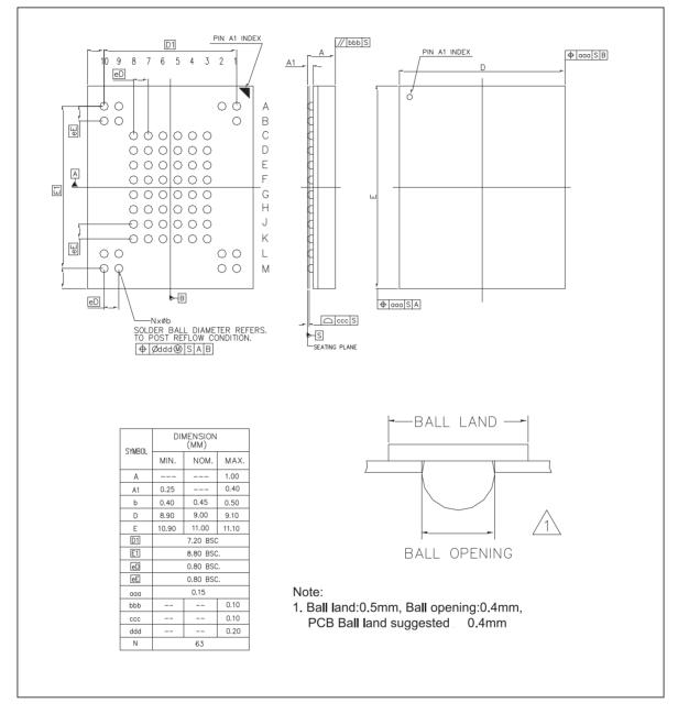
Figure 13-2 Fine-Pitch Ball Grid Array 63-Ball
