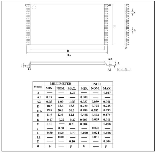
Figure 13-1 TSOP 48-pin 12x20mm
