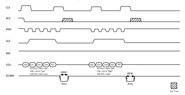
Figure 9-19 Two Plane Block Erase Operation
