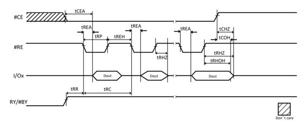
Figure 11-4 Serial Access Cycle after Read
