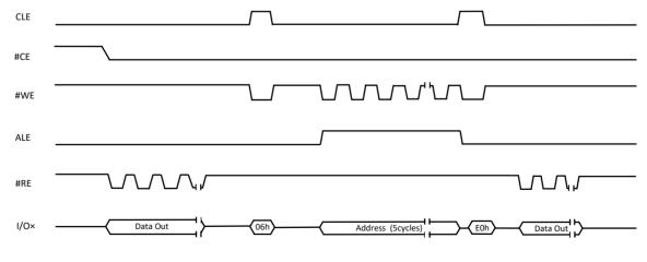
Figure 9-4 Two Plane Random Data Read (06h-E0h) Operation
