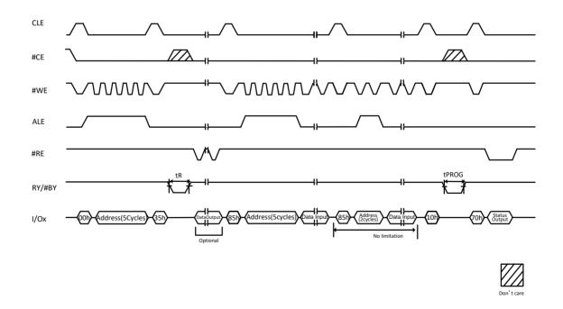
Figure 9-14 Copy Back Operation with Random Data Input
