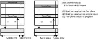
Figure 9-17 Two Plane Program for Copy Back
