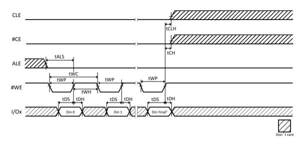
Figure 11-3 Data Latch Cycle
