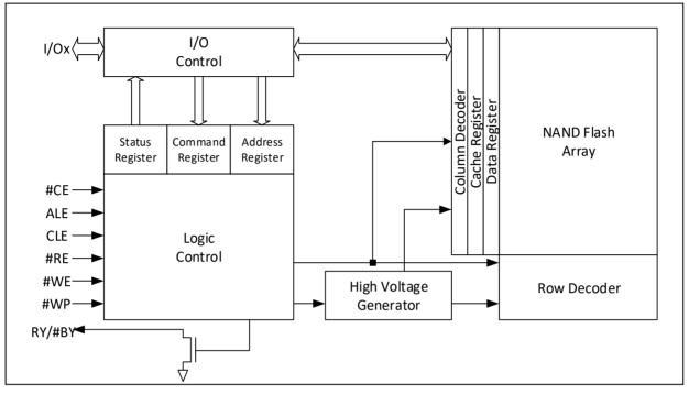
Figure 5-1 NAND Flash Memory Block Diagram
