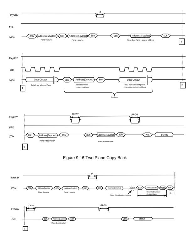
Figure 9-16 Two Plane Copy Back with Random Data Input
