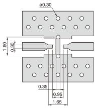
Line width should be designed to match  $50\Omega$  characteristic impedance, depending on PCB material and thickness.
