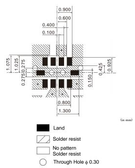
$\mbox{\%}\,\square$  Line width to be designed to match 50  $\Omega$  -characteristic impedance, depending on PCB material and thickness.
