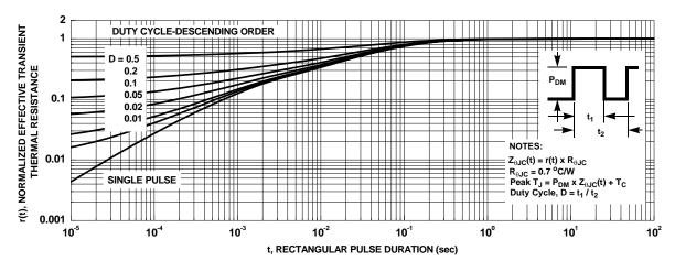
Figure 15. Junction-to-Case Transient Thermal Response Curve for FDP2D3N10C
