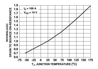
Figure 3. Normalized On-Resistance vs. Junction Temperature
