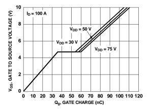
Figure 7. Gate Charge Characteristics
