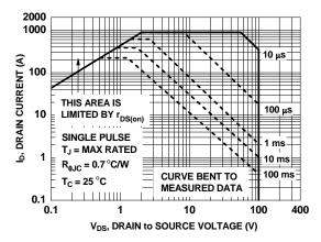
Figure 11. Forward Bias Safe Operating Area for FDP2D3N10C
