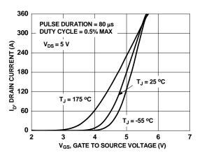
Figure 5. Transfer Characteristics
