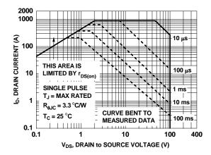
Figure 12. Forward Bias Safe Operating Area for FDPF2D3N10C
