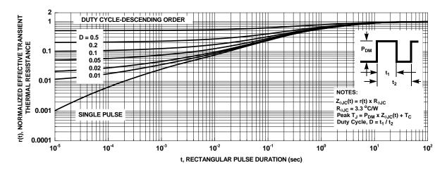
Figure 16. Junction-to-Case Transient Thermal Response Curve for FDPF2D3N10C
