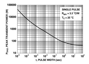
Figure 13. Single Pulse Maximum Power Dissipation for FDP2D3N10C
