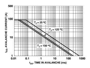
Figure 9. Unclamped Inductive Switching Capability
