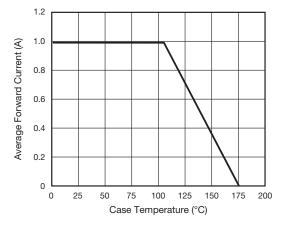
Fig. 1 - Forward Current Derating Curve
