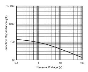
Fig. 4 - Typical Junction Capacitance
