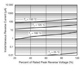
Fig. 3 - Typical Reverse Characteristics
