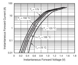
Fig. 2 - Typical Instantaneous Forward Characteristics
