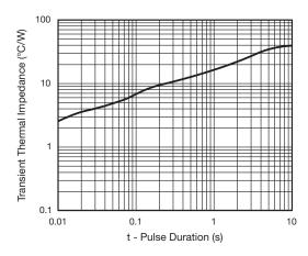
Fig. 5 - Typical Transient Thermal Impedance
