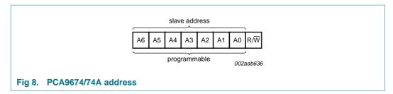
The last bit of the first byte defines the operation to be performed. When set to logic 1 a read is selected, while a logic 0 selects a write operation.
