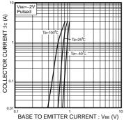
Fig.4 Grounded emitter propagation characteristics
