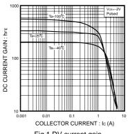
Fig.1 DV current gain vs. collector current
