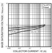
Fig.3 Base-emitter saturation voltage vs. collector current
