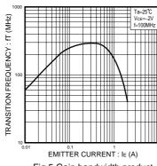
Fig.5 Gain bandwidth product vs. emitter curent
