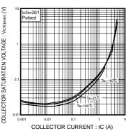
Fig.2 Collector-emitter saturation voltage vs. collector current
