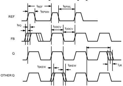
Figure 4. Zero Skew and Zero Delay Clock Driver
