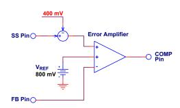
Figure 2: The A8589 Error Amplifier
