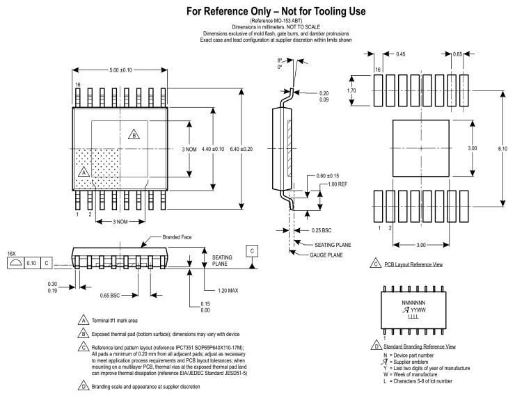
Figure 28: Package LP, 16-Pin TSSOP with Exposed Thermal Pad
