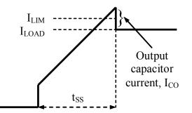
Figure 19: Output Current (I<sub>CO</sub>) During Startup
