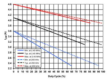
Figure 11: Pulse-by-pulse Current Limiting versus Duty Cycle; at f<sub>SW</sub> = 250 kHz (dashed curves) and f<sub>SW</sub> = 2.45 MHz (solid curves)
