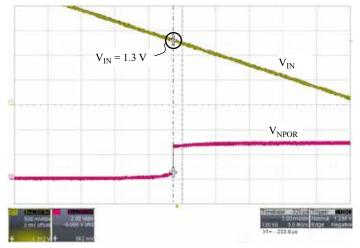
Figure 10: NPOR being Held Low as V<sub>IN</sub> Ramps Down
