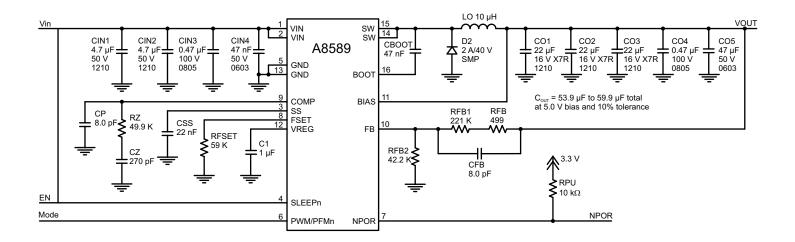
Figure 27: Typical Application Schematic B. Configured for V<sub>IN</sub> = 12 V, V<sub>OUT</sub> = 5.0 V, I<sub>OUT</sub> = 2.5 A at 425 kHz
