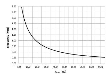
Figure 17: PWM Switching Frequency versus R<sub>FSET</sub>
