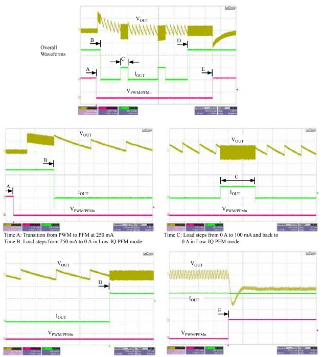
Time D: Load steps from 0 A to 250 mA in Low-IQ PFM mode
