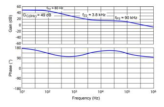
Figure 21: Type-II Compensated Error Amplifier
