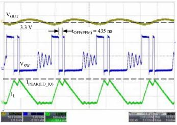
Figure 5. Low-IQ PFM Mode Operation at V<sub>IN</sub> = 12 V, V<sub>OUT</sub> = 3.3 V, and I<sub>OUT</sub> = 330 mA. SW turns on only twice every 5  $\mu$ s to regulate V<sub>OUT</sub>
