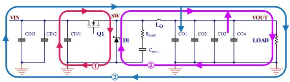
Figure 24: Typical B uck Converter with Critical Paths/Loops Shown
