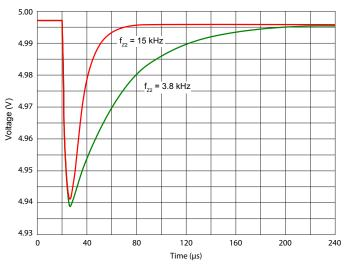
Figure 23: Transient Recovery Comparison for f<sub>Z2</sub> at 3.8 kHz/69° and 15 kHz/60°
