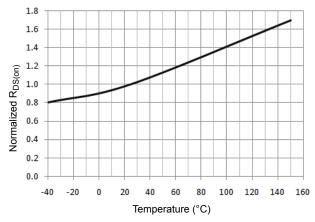
Figure 3: Typical MOSFET R<sub>DS(on)</sub> versus Temperature
