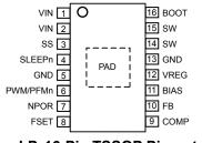
Package LP, 16-Pin TSSOP Pin-out Diagram
