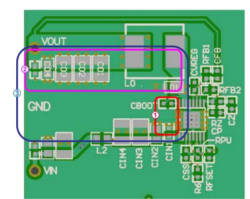
Figure 25: Example PCB Component Placement and Routing
