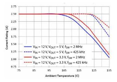
Figure 1: A8589 Typical Current Derating
