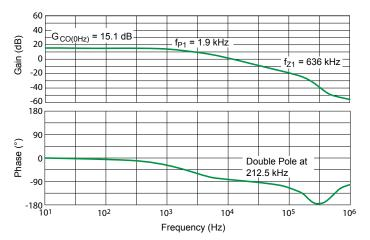
Figure 20: Control-to-Output Bode Plot
