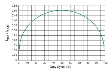
Figure 18: Input Capacitor Ripple versus Duty Cycle
