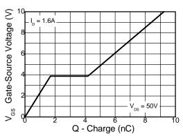
Gate-Source Voltage v Gate Charge
