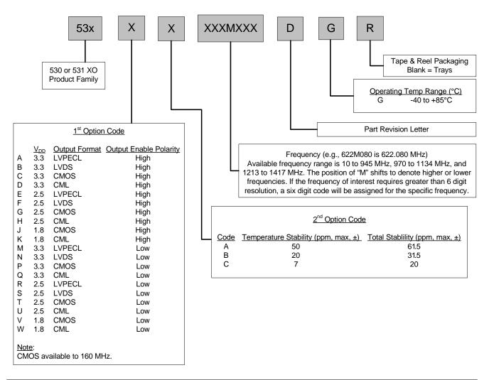
Example P/N: 530AB622M080DGR is a 5 x 7 XO in a 6 pad package. The frequency is 622.080 MHz, with a 3.3 V supply, LVPECL output, and Output Enable active high polarity. Temperature stability is specified as  $\pm 20$  ppm. The part is specified for -40 to  $\pm 85$  °C ambient temperature range operation and is shipped in tape and reel format.
