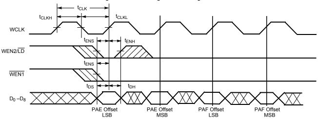
Figure 15. Read Programmable Registers
