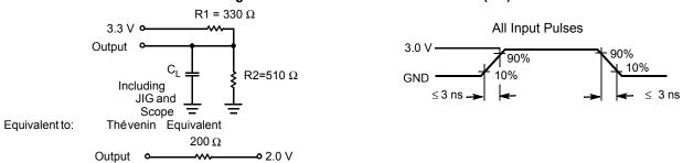
Figure 5. AC Test Loads and Waveforms (-10)
