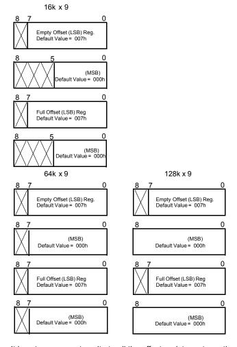
It is not necessary to write to all the offset registers at one time. A subset of the offset registers can be written; then by bringing the WEN2/LD input HIGH, the FIFO is returned to normal read
