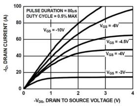
Figure 8. Saturation Characteristics
