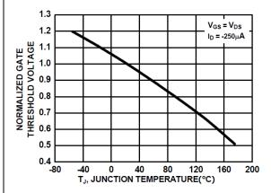
Figure 11. Normalized Gate Threshold Voltage vs.
