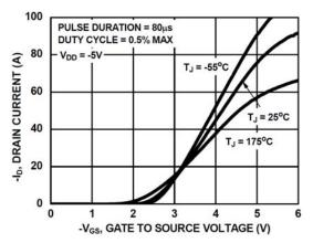
Figure 7. Transfer Characteristics
