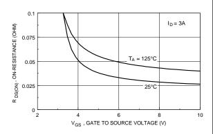
Figure 3. On-Resistance Variation with Temperature.
