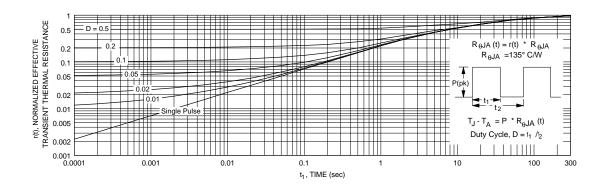
Figure 11. Transient Thermal Response Curve.
