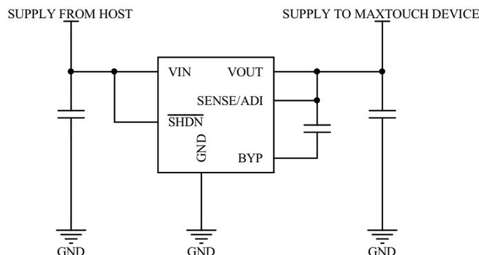
An LDO regulator should be chosen that provides adequate output capability, low noise, good load regulation and step response. The voltage regulators listed in Table 10-1 have been tested and found to work well with maXTouch devices. If it is desired to use an alternative LDO, however, certain performance criteria should be verified before using the device. These are:
