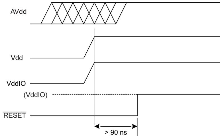
Note: When using external  $\overline{\text{RESET}}$  at power-up, VddIO must not be enabled after Vdd
