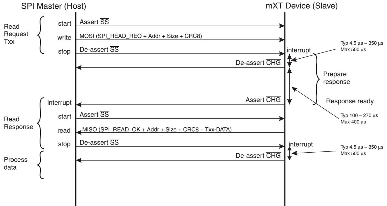
Normally a limit of 64 bytes is allowed for data reads. If the host tries to read more than 64 bytes, the slave returns SPI\_READ\_FAIL (see [Section 9.4.3 “SPI\\_READ\\_FAIL”](#)). A mechanism is provided, however, that supports the DMA transfer of a large block of data that exceeds this limit. This is achieved by the provision of multiple instances of the Data Container T117 object within the device that allow up to 1290 bytes of data to be read in a contiguous manner.
