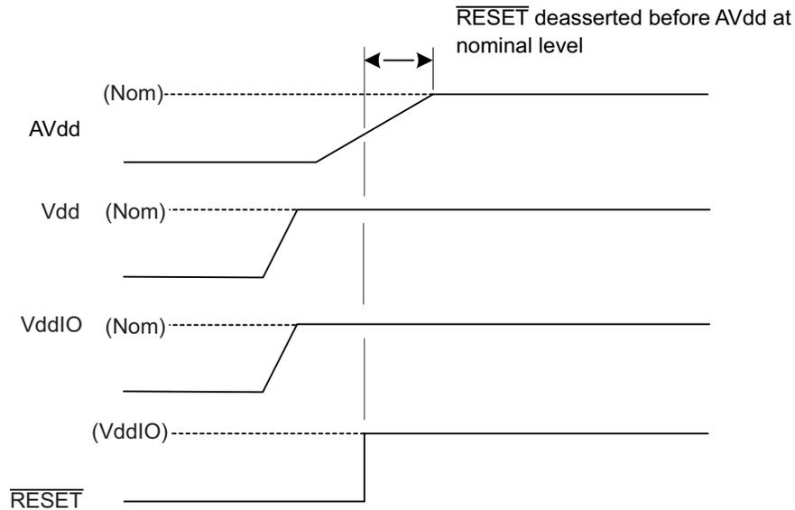
The  $\overline{\text{RESET}}$  pin can be used to reset the device whenever necessary. The  $\overline{\text{RESET}}$  pin must be asserted low for at least 90 ns to cause a reset. After releasing the  $\overline{\text{RESET}}$  pin the device typically takes 90 ms before it is ready to start communications. It is recommended to connect the  $\overline{\text{RESET}}$  pin to a host controller to allow it to initiate a full hardware reset without requiring a power-down.
