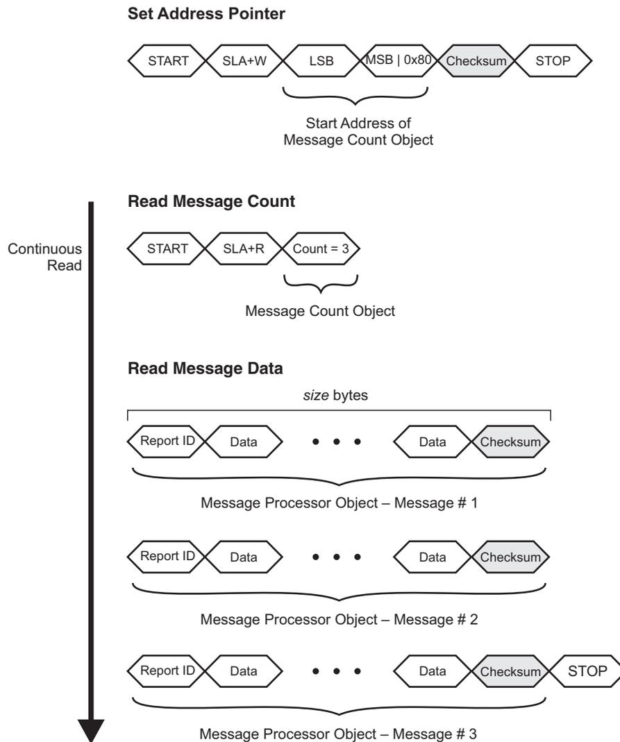
There are no checksums added on any other I<sup>2</sup>C reads. An 8-bit CRC can be added, however, to all I<sup>2</sup>C writes, as described in [Section 8.3 “I<sup>2</sup>C Writes in Checksum Mode”](#).
