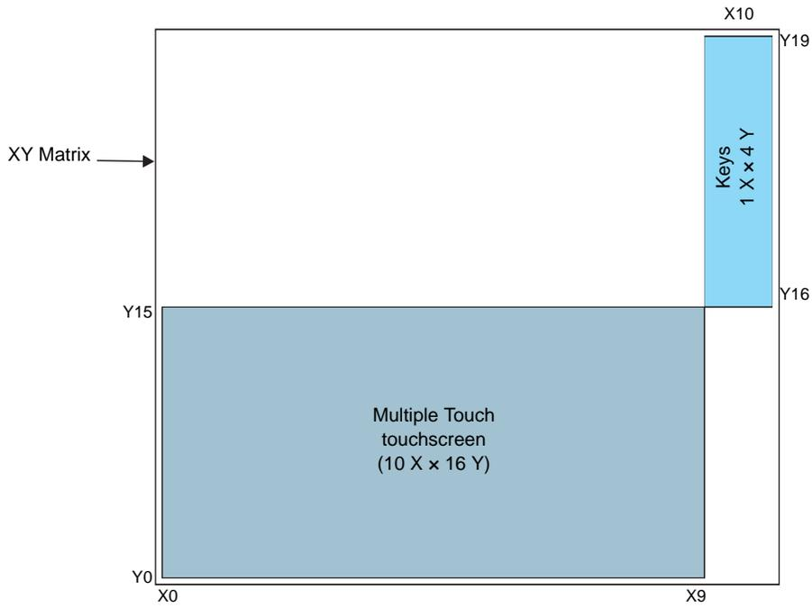
If, however, the intention is to preserve a larger touchscreen size and maintain an optimal aspect ratio, then using equal X and Y lines for the key array can be considered, as in [Figure 4-2](#).
