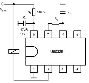
Figure 2-2. Basic Circuit for V<sub>S</sub> = 5V
