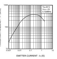
Fig.5 Gain bandwidth product vs. emitter current
