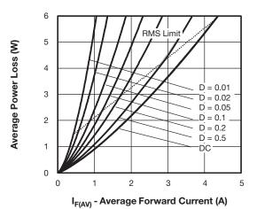
Fig. 5 - Forward Power Loss Characteristics
