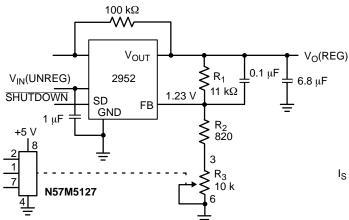
Figure 7. Programmable Voltage Regulator
