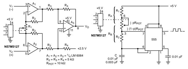
Figure 5. Programmable Instrumentation Amplifier
