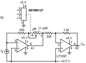
Figure 8. Programmable I to V Convertor
