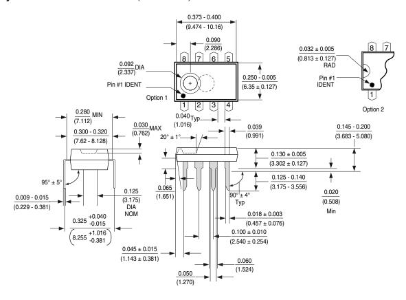
Molded Dual-In-Line Package (N) Package Number N08E
