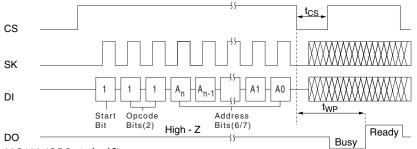
93C46A (ORG=1;  $A_n$ =A5): Address bits pattern -> A5-A4-A3-A2-A1-A0; User defined 93C46A (ORG=0; A<sub>n</sub>=A6):
