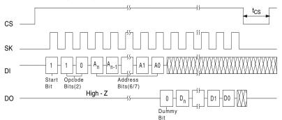
93C46A (ORG=1;  $A_n$ =A5;  $D_n$ =D15): Address bits pattern -> A5-A4-A3-A2-A1-A0; User defined 93C46A (ORG=0;  $A_n$ =A6;  $D_n$ =D7): Address bits pattern -> A6-A5-A4-A3-A2-A1-A0; User defined
