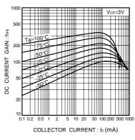
Fig.5 DC current gain vs. collector current
