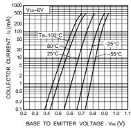
Fig.1 Grounded emitter propagation characteristics
