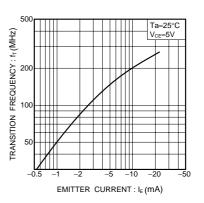
Fig. 6 Gain bandwidth product vs. emitter current
