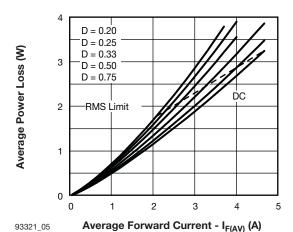
Fig. 5 - Forward Power Loss Characteristics
