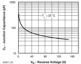
Fig. 3 - Typical Junction Capacitance vs.
